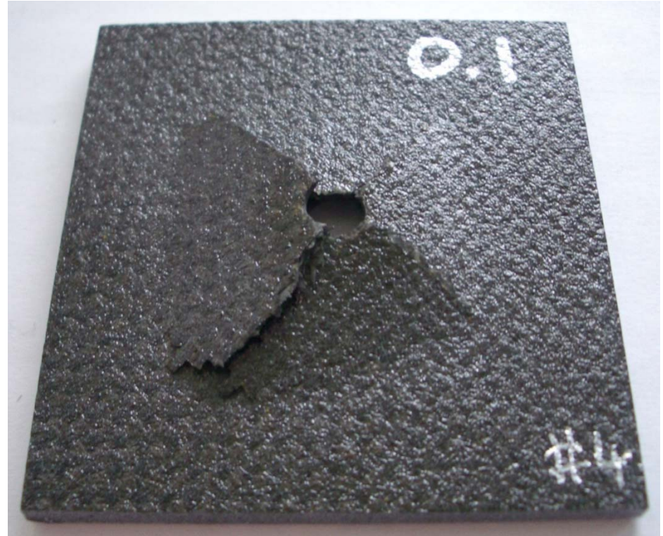
Pull-through failure (above)
